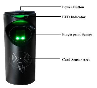
LED indicator: The LED indicator is used to display device operation results and exceptional statuses which are defined as follows:
